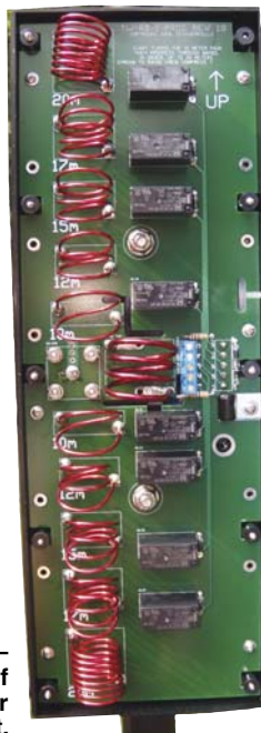
Figure 2 — Interior view of the Adventurer matching unit.
